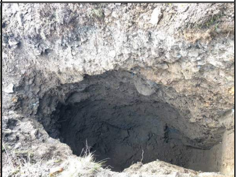
Exposed subsurface soil profile within test-pit TP-3
