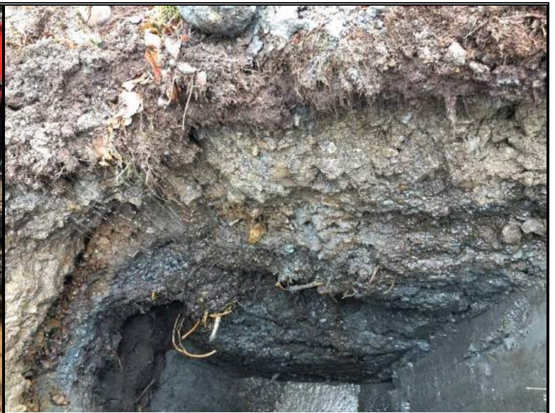
Exposed subsurface soil profile within test-pit TP-1
